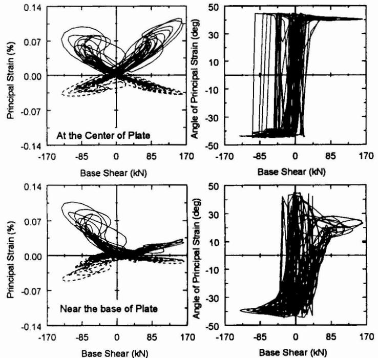
Figure 6: Magnitude and angle of principal strains at the centre and near the base of the first storey infill plate for Tarzana 140% run
