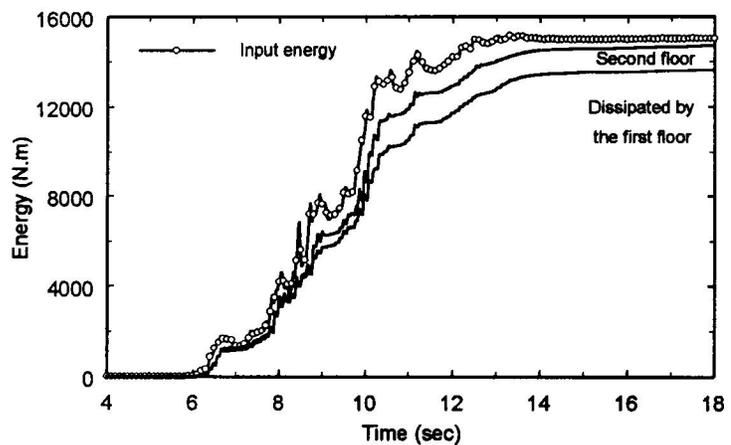
Figure 5: Input energy together with the first and second floor dissipated energy time-histories for Tarzana 140% test
