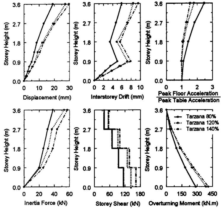
Figure 4: Maximum response envelopes of the test specimen for Tarzana Hill runs
