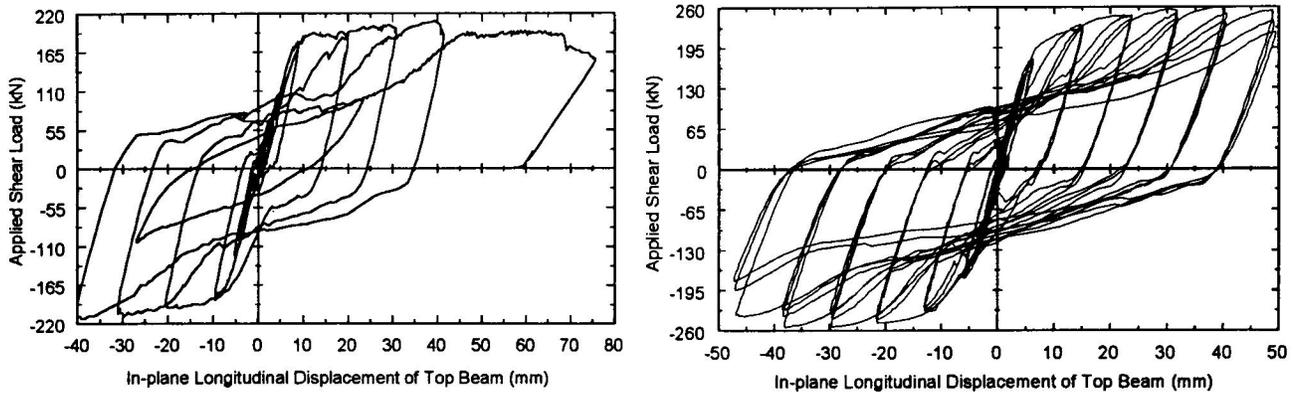
Figure 2: Hysteresis curves of the first (left) and second (right) single storey shear wall specimens
