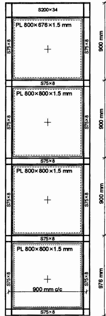
Figure 1: Four-storey steel plate shear wall specimen
