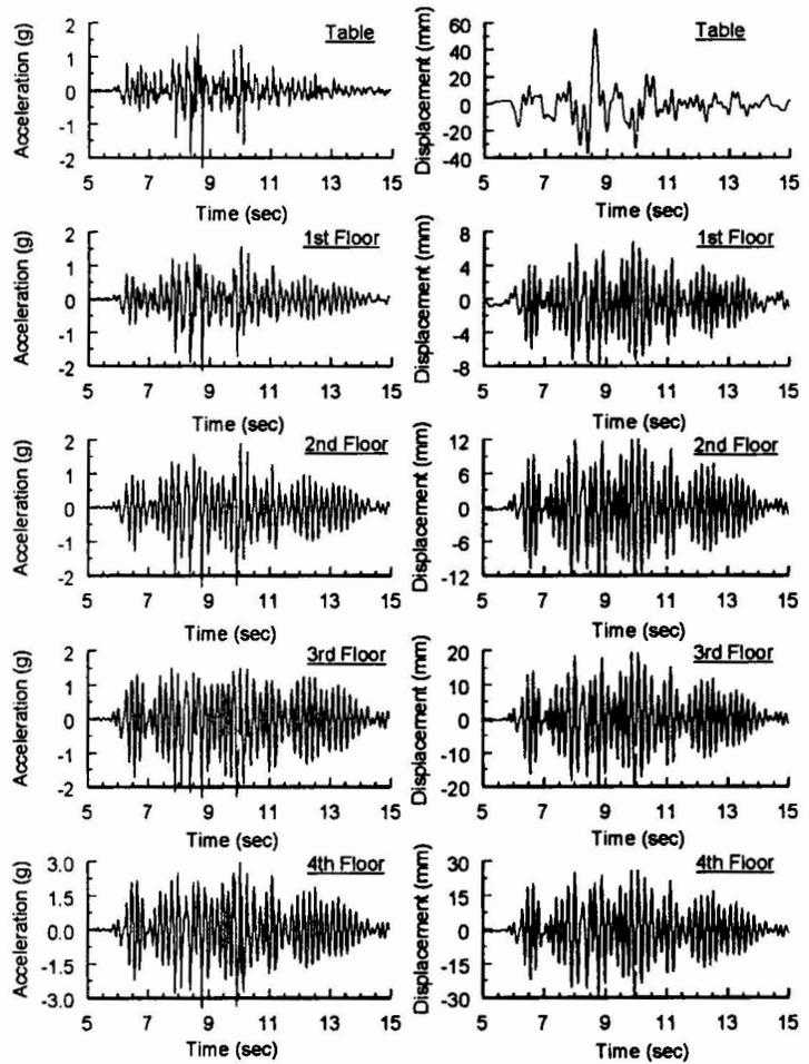
Figure 3: Time-histories of the table and floor accelerations, table displacement and floor relative displacements for Tarzana 140%
